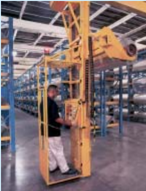
Roll Storage with Man Aboard Stationary Cab
