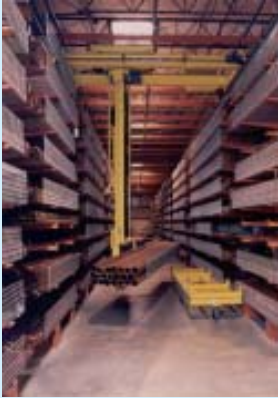
Copper Tube Storage System on Cantilever Rack
