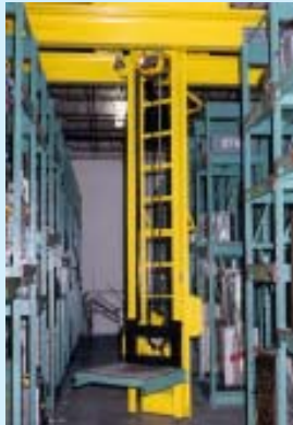
Stacker Crane Retrofit to Existing Racking System
